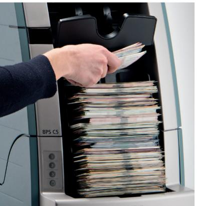
The large feeder holds up to 1,500 banknotes, ensuring a continuous workflow
